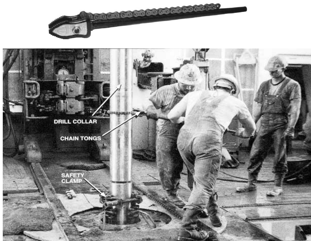
Figure 106 Chain tong and usage on rig floor
